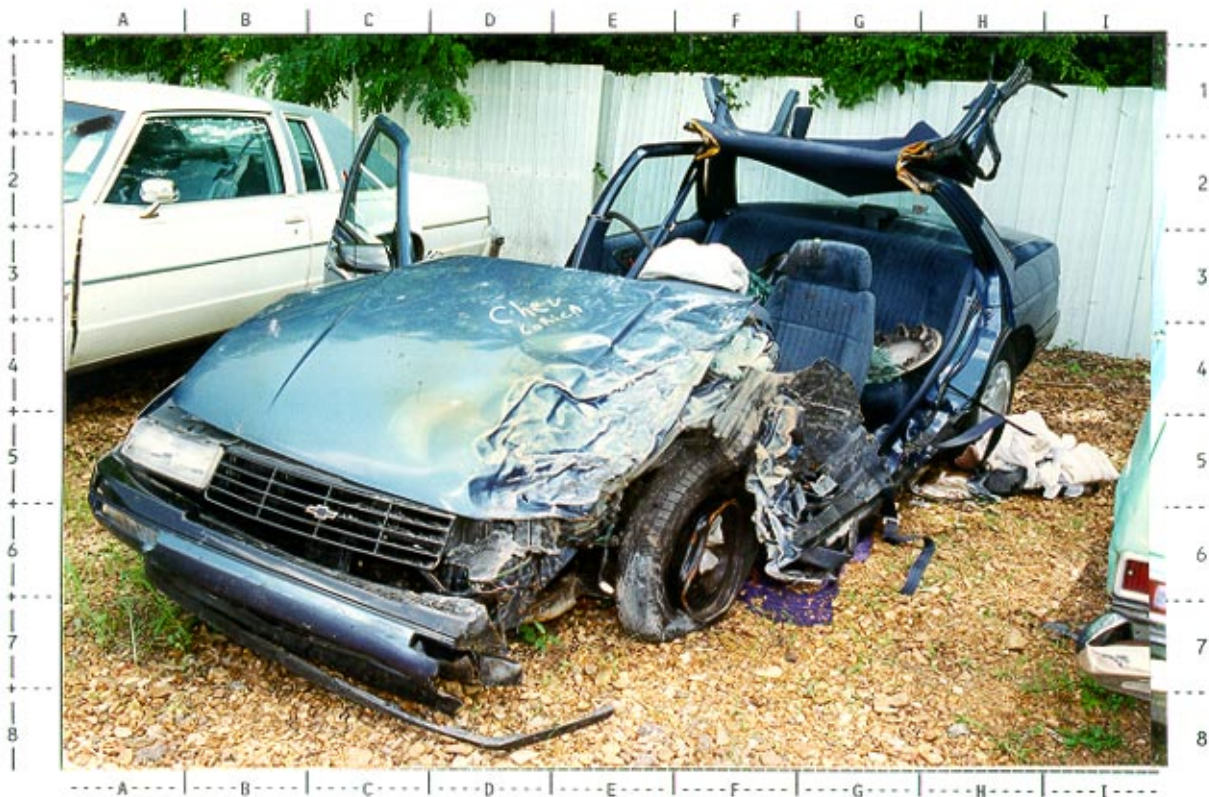
# 32 -- Front left (45 degree angle) view of 1991 Corsica's front left damage without contour gauge present; NOTE: roof & cut pillars
